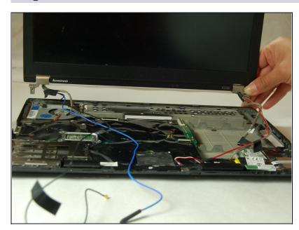
Carefully lift the screen module straight up to detach from board.
