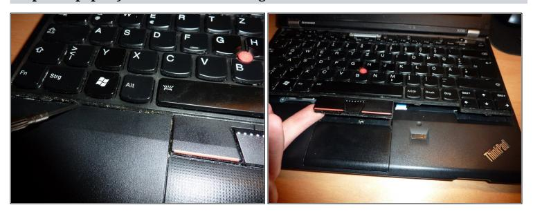
• Use a a plastic spudger (or a flat screwdriver) to push the keyboard towards the screen. This will pop the bottom of the keyboard out of the casing.
