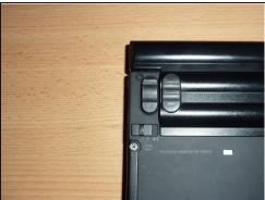
• Locate the two switches that lock the battery. Push the left-hand switch outward into the "unlocked" position.
