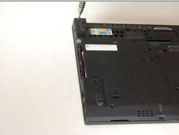
• Unscrew two 5.7mm screws from the top of the bottom of the laptop.
