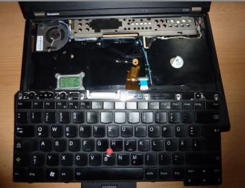
• Carefully lift the keyboard so that you can access its connector.
