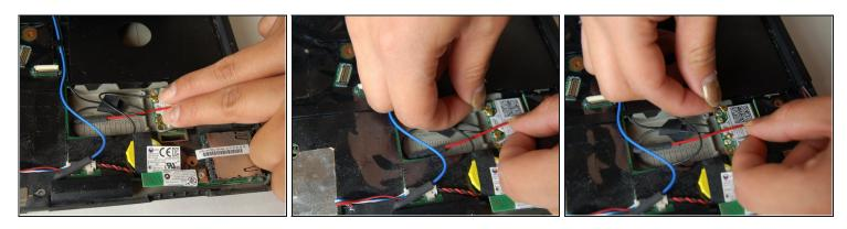
• Carefully disconnect blue and red cables and remove them from plastic case.
