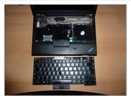
You are done - the keyboard is not connected to the laptop any more and can be replaced.
