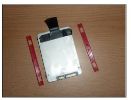
• Remove the plastic rails from the old SSD/hard drive and place them on the new SSD/hard drive.
