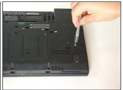
• Remove five 5.7mm screws from the bottom.
