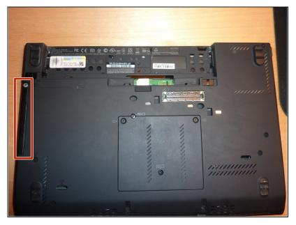
Locate the hard drive enclosure (marked by the red rectangle).
