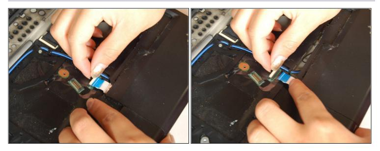
• Unlock the white seal and disconnect the blue cable.
