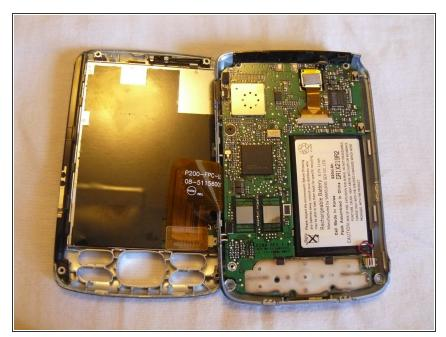
Pull the back panel off the body of the unit to expose the motherboard in the body.
