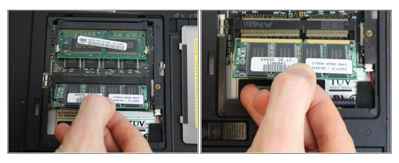
Using your fingers, pull straight in line with the ram to remove it.
