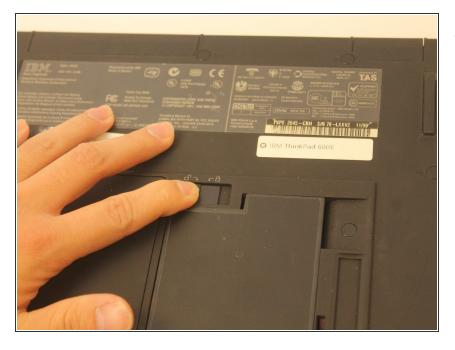
Move the latch to the side with the unlocked symbol.
