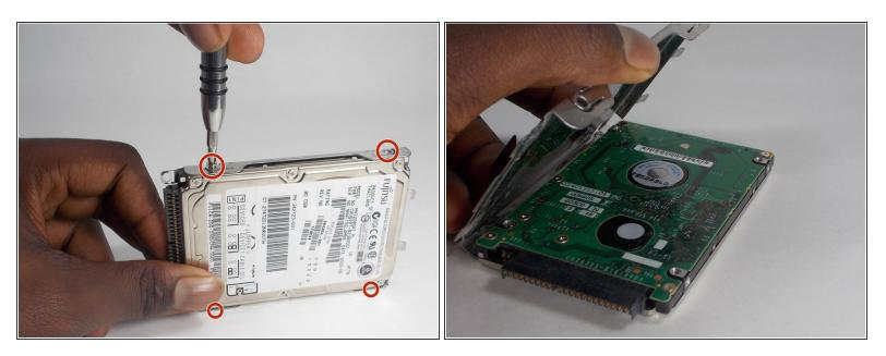
Remove the four 4mm Philips #1 screws, two on each side, that secure the hard drive frame to the hard drive.
