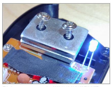
Remove 2 screws to lift-up the two metal weights
