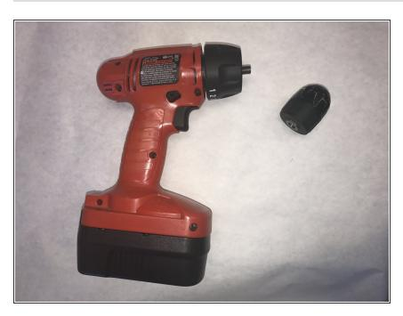
Remove the chuck completely by unscrewing it in a counter clockwise direction.
