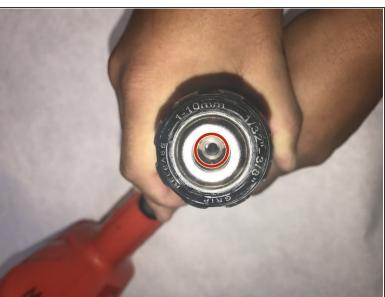
Using the T20 Torx Security screwdriver, take out the 2.3 mm screw inside the chuck.
