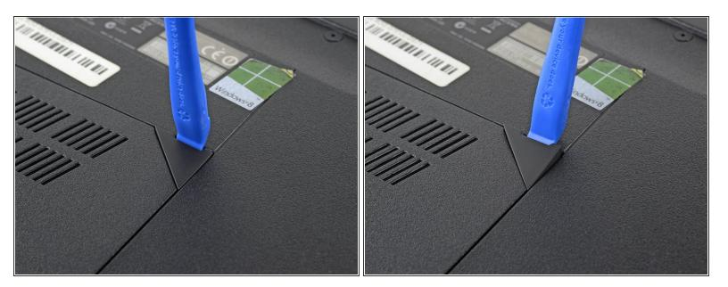
Use an opening tool to pry up the small rubber cover on the upper right corner of the RAM access door.
