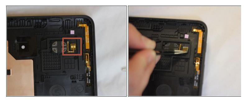
Locate the speaker in the top right corner of the back casing. Use a pair of tweezers to pull peel up the film connecting the speaker to the case.
