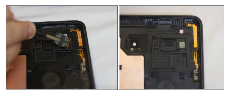
• Once you've detached the film connecting the speaker to the case, use the tweezers to remove the speaker completely.
