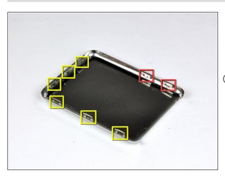
The rear panel is secured to the front case by eight clips permanently attached to the rear
