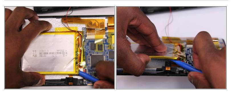
Using a spudger, gently pry the battery from the back of the screen to remove it from the device.
