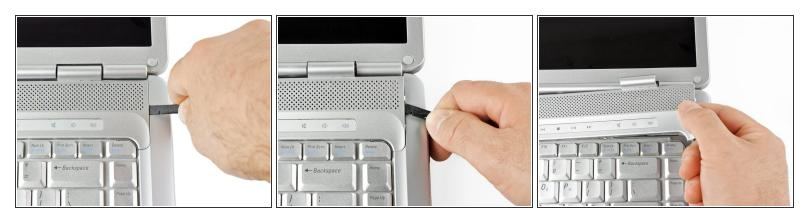
Insert the flat end of a spudger into the slot on the right side of the central control cover and pry it up.
