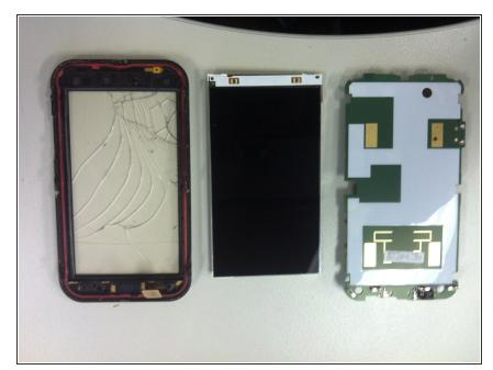
Separate the Frame + Digitizer, the LCD and the mainboard.
