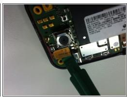
After opening the device, carefully, using the plastic opening tool, peel off the lcd and digitalizer conectors from the mainboard.
