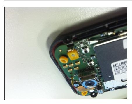
Remove the two yellow rubber protectors near the screws. The rectangular yellow rubber protector might fall off too so put it aside.
