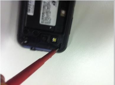
Using a Torx T5 screwdriver, remove both screws near the camera.
