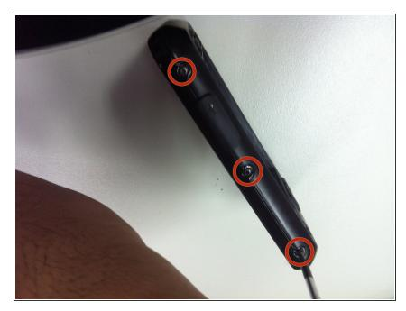
Using the Torx T5 screwdriver, remove all 7 screws around the mobile: 3 on each side + 1 on the botton.
