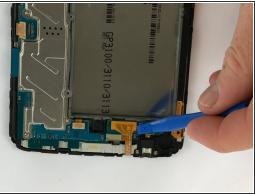
Disconnect all the flex cables from the motherboard by prying the connectors straight up.
