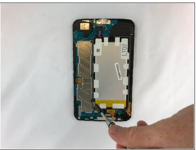
Remove the ten 4 mm Phillips #000 screws securing the motherboard.
