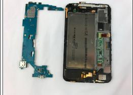
Remove the motherboard from the device by carefully lifting it out.
