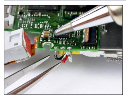
All leads should now be desoldered and disconnected from the logic board.
