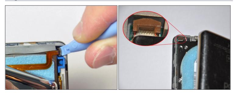
• Use angled tweezers or an iPod opening tool to slide up the brown connector latch, holding the orange battery ribbon cable in place. Make sure you pull from both sides of the latch. You only need to lift the brown connector latch up about 1-2mm to free the cable. Do not lift more or remove the latch, or you might pull the white connector with it!
