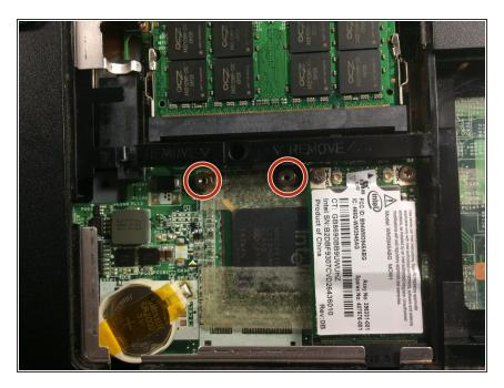
Using the size 5.0mm hex tool, unscrew the 2 brass screws located near the RAM cards under the laptop.
