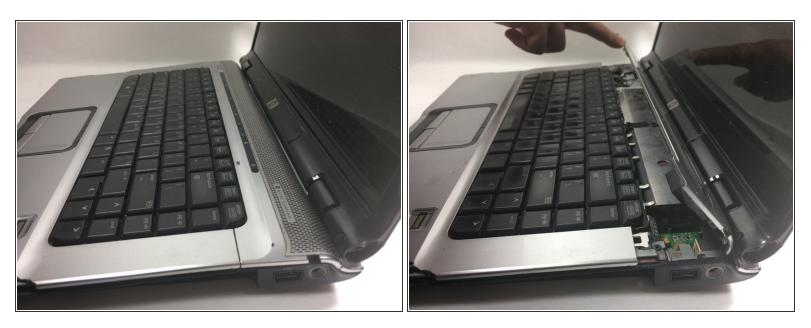
• Gently lift the plastic panel on the top of the laptop at the divide until the two ribbon cables and cable leads are visible with their ports on left side on laptop.
