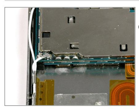
The solder bead should look like a small dome or hemisphere. If it is flat or jagged, simply place the soldering iron back on the solder to re-melt it and then pull the soldering iron away. It may require a little more solder if this does not work.
