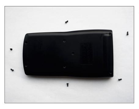
Place the back side of the casing back on top of the front.
