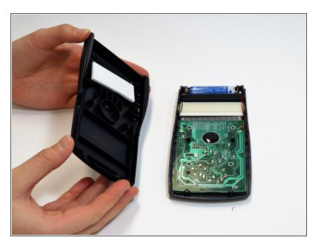
Once all six screws have been removed, take the back part off of the calculator.
