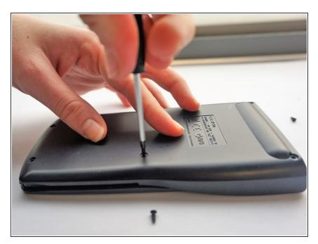
Put all six screws back in the back side of the casing.
