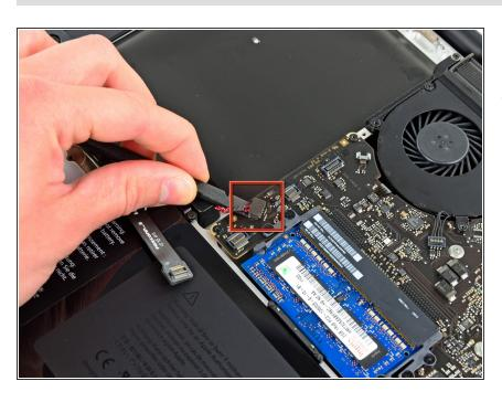
Using the flat end of a spudger, pry the subwoofer connector straight up off the logic board.
