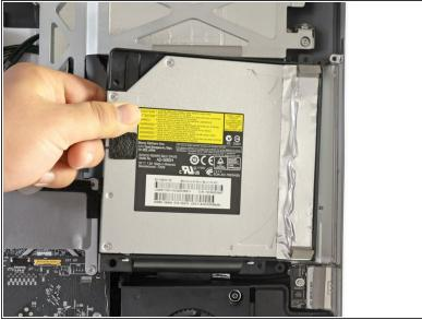
Slightly lift the left edge of the optical drive and then pull it to the side to release the centering pins.
