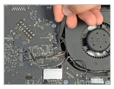
Use the tip of a spudger to pull the optical drive thermal sensor connector out of its socket.
