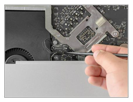
Use the flat edge of a spudger to release the CPU fan cable
