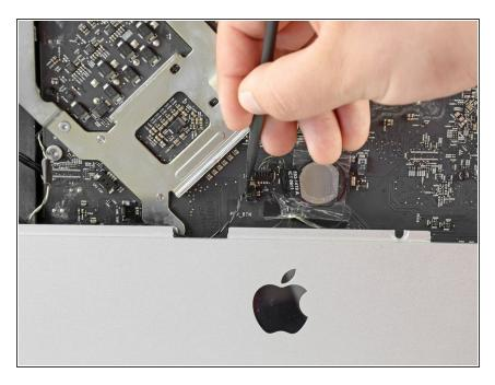
Use the flat edge of a spudger to pull the power button connector free of its socket.
