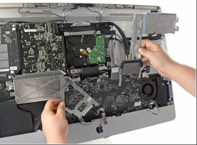
Simultaneously lift and rotate the logic board and heat sink assembly away from the iMac case until you can easily access the back side of the logic board.
