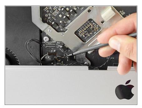
Use the flat end of the spudger to push the ambient temperature sensor connector out of its socket.
