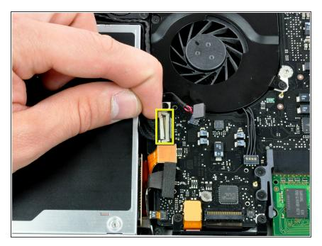
Disconnect the camera cable by pulling the male end straight away from its socket.
