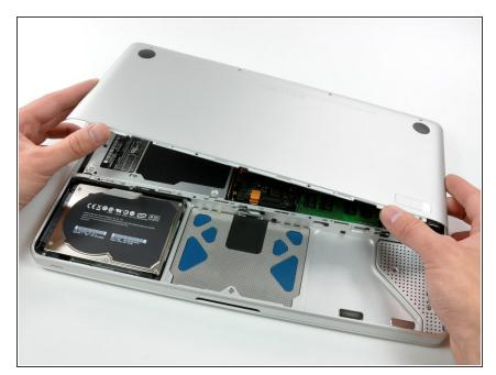
Using both hands, lift and remove the lower case off the upper case.
