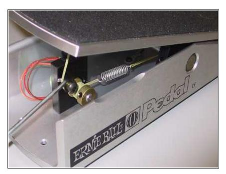
Pull the long cord forward and onto the front black pulley. Make sure that the short cord is in place on the back black pulley.
