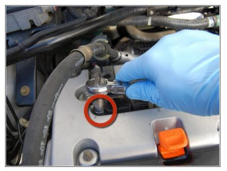
• Using the 10mm socket and ratchet, remove the 4 bolts holding down the coilpacks. You may need the 10mm wrench if your socket is not deep enough to contact the hex section of the stud.
