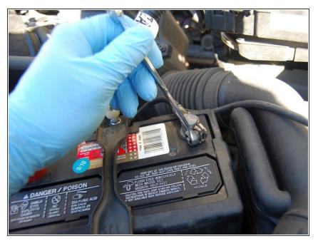
• Reinstall the negative (-) battery terminal, tightening with the 10mm wrench or 10mm ratchet.
