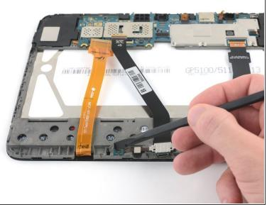
Use the flat end of a plastic spudger to gently pry the press-fit connector from the microphone's ribbon cable.
