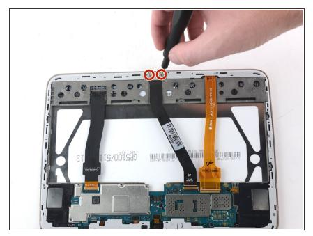
Use a Phillips #000 screwdriver to remove the two 3mm screws in the metal plate connecting the charging port to the display assembly.
