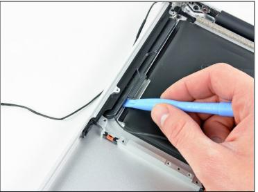
• Use a plastic opening tool or another thin prying object to carefully pry the right speaker up from the adhesive securing it to the upper case.
