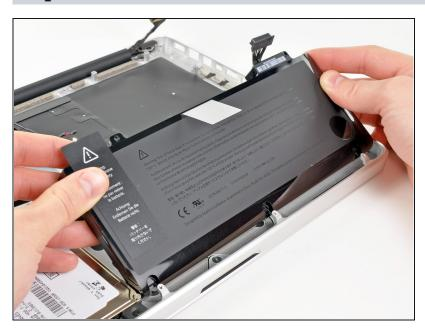
Use the attached plastic pull tab to help remove the battery from the upper case.
