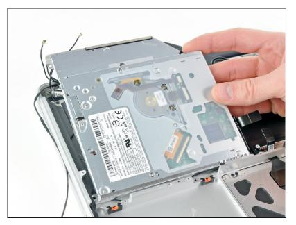
Lift the optical drive from the edge nearest the display and remove it from the upper case.
