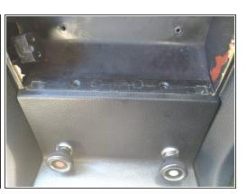
Now you can remove those two counter-sunk screws holding in the front of the shifter/center console panel.
