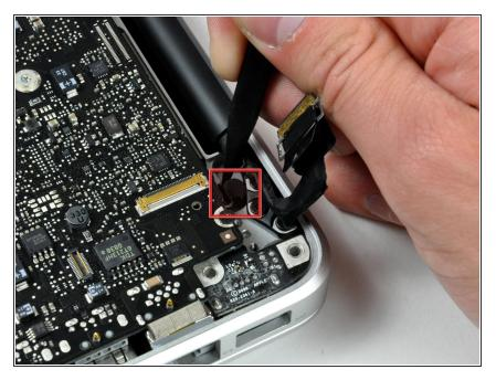
• Use the tip of a spudger to release the microphone from the upper case.
