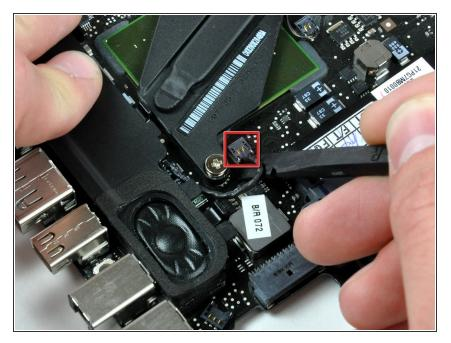
Use the flat end of a spudger to pry the left speaker connector up off the logic board.
