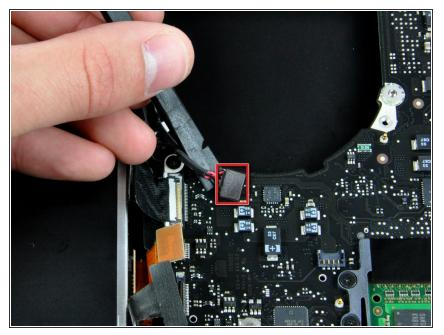
• Use the flat end of a spudger to pry the subwoofer cable connector straight up off the logic board.
