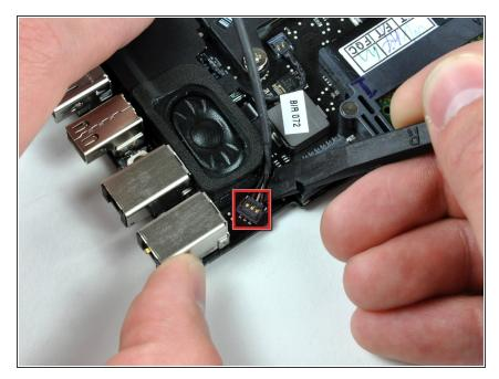
• Use the flat end of a spudger to pry the microphone cable connector up off the logic board.
