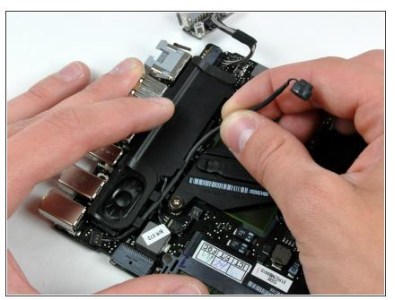
• Deroute the microphone cable from the channel in the left speaker.
