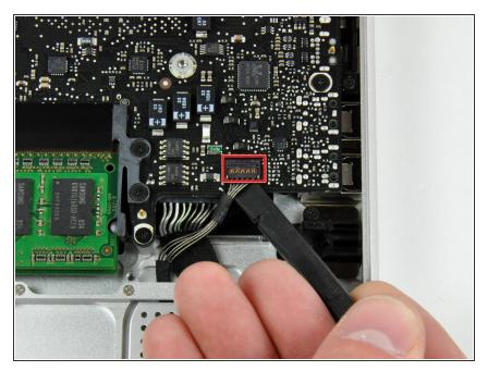
• Use a spudger to pry the battery level indicator cable connector straight up off the logic board.
