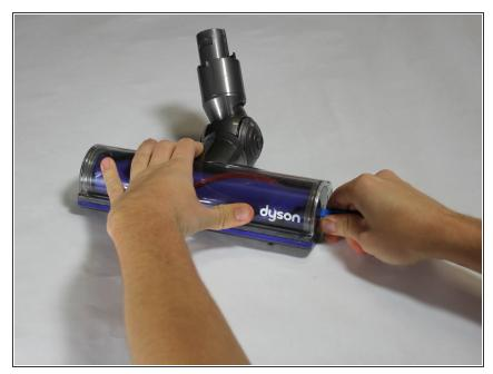
• Turn the end cap counterclockwise using the iFixit Opening Tool.
