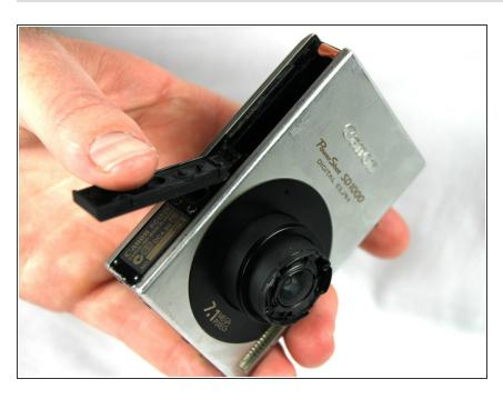
Let the battery cover open fully and rest as shown.
