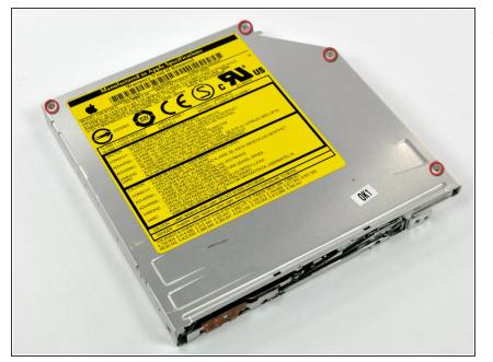
With the optical drive removed from the computer, remove the screws securing the top panel of the optical drive.
