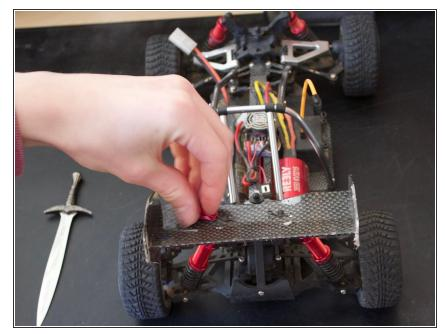
i TIP: If the component is often removed (for example, for thorough cleaning), it is helpful to provide the splints with some insulating tape, so tools are unnecessary
