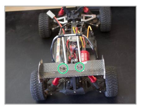
These two pins must be removed
