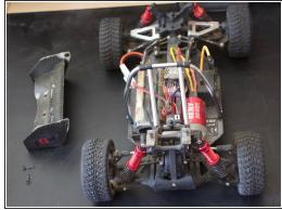
After that, the spoiler can be removed upwards
