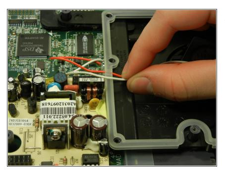
Remove the red and white wires from the rubber casing rim.
