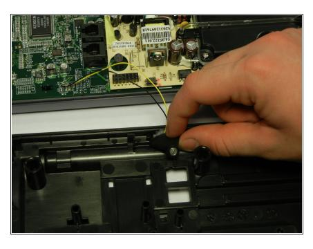
Disconnect the rubber piece by pulling it out of the slot, freeing the back cover completely.
