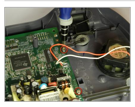
Remove the two 8mm Phillips #2 screws.
