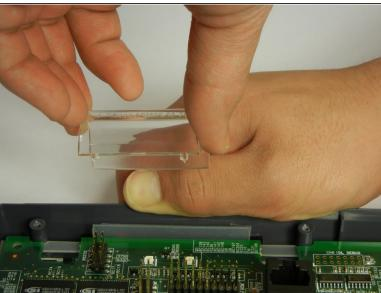
Pull the gray plastic casing away from the circuit board as you remove the clear, curved, plastic piece straight up.
