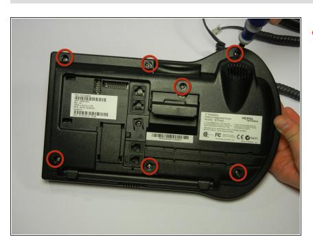
Remove the seven 8mm Phillips #2 screws.
