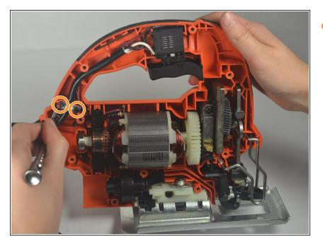
Remove the two 12.7mm phillips head screws holding the power cord in place with a PH2 Phillips head screwdriver.
