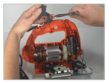
Remove the two 6.35mm flat head screws on the trigger with a 2.5 flat head screwdriver to disconnect the white and black cords.
