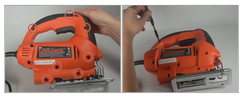
• Remove the nine torx 15.875mm screws on the front of the jigsaw using a T-15 torx screwdriver.
