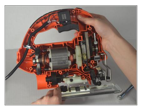
• Simply remove the shoe plate by pulling it down and out.
