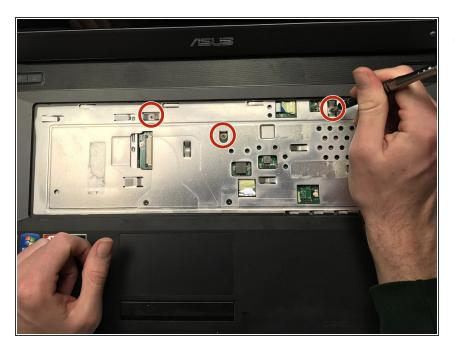
Remove the 4mm screws located under the keyboard with the PH0 screwdriver.
