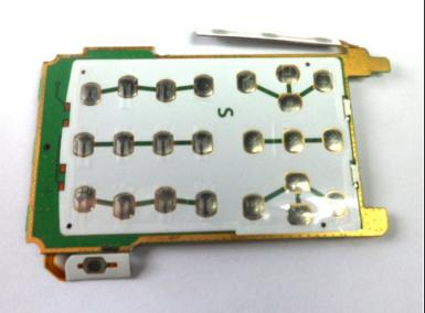
Pull the two boards apart to separate the keypad from the motherboard.
