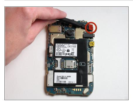
Using a spudger, lift the ribbon band in the upper right-hand corner up and away from the motherboard assembly until it disconnects.
