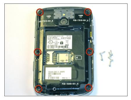
Remove the six 7.0mm Torx screws securing the rear case to the rest of the phone.
