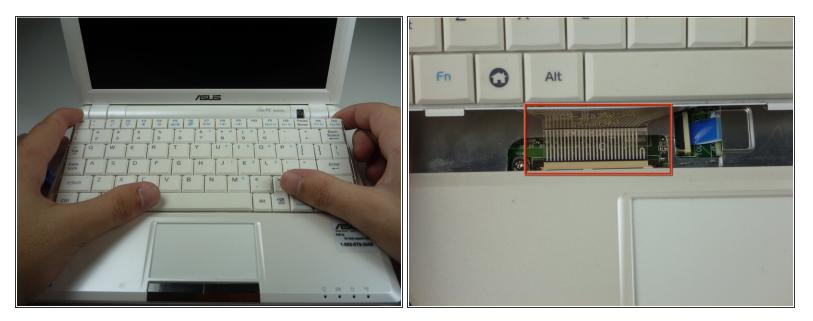
Clips hold the bottom portion of the keyboard to the laptop. Gently lift the upper portion of the keyboard and then move the entire keyboard towards the computer's screen until the ribbon cable is visible.
