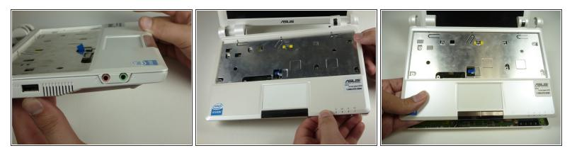
**Caution:** To clear the audio and microphone, lift the right half and move the cover to the left (as shown in the second picture) to prevent cover damage.
