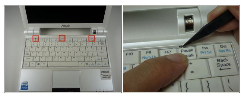
Caution Follow this step to detach the upper portion of the keyboard, but do not remove it from the laptop. Damage to the keyboard's ribbon cable may result if improperly executed.
