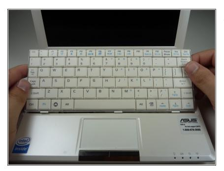
Remove the keyboard by lifting upwards.
