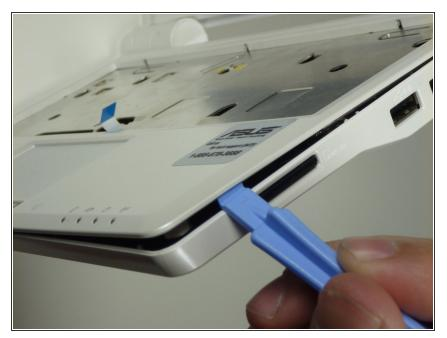
• Use a plastic opening tool to gently detach the top cover from the laptop's base. See the next step for removing the cover.
