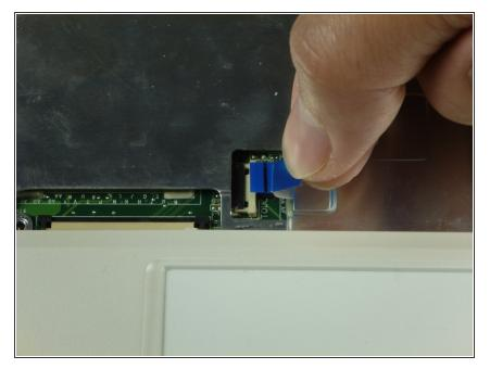
Slide out the touchpad's ribbon connector by pulling the blue tab to the right.
