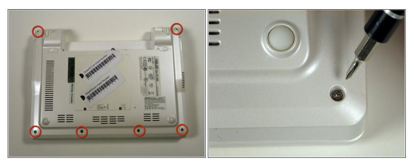
Remove the six 4.76 mm Phillips #0 screws on the back of the laptop.
