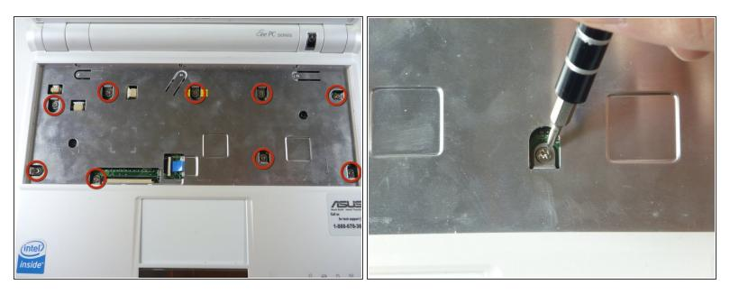
Remove the nine 4.76mm Phillips #0 screws on the top cover of the laptop.
