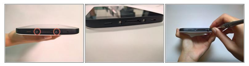
• Using a Tri-Point YO Screwdriver, remove the two 4.1mm Tri-Wing screws.
