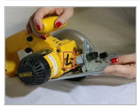
Take out the Allen Key that is located on the front of the saw below the smooth control handle on the top of the saw.
