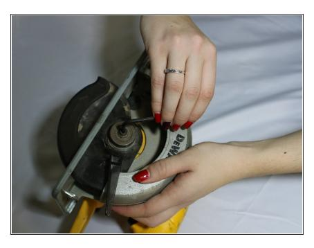
Use the Allen Key to replace to loosen the bolt where the center of the saw is/would be.
