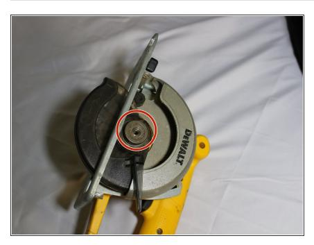
Remove the circular nut that is used to hold the saw blade in place. It slide right off.
