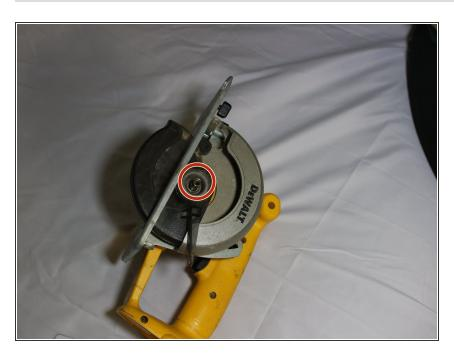
Place blade on the peg in the middle of the saw. The peg has two flat sides as does the saw hole to prevent slipping when spinning.
