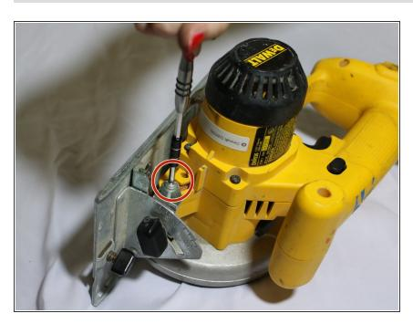
Using an H 4.0 hex head screw, unscrew the bolt located right above the boot that is next to the motor of the saw.
