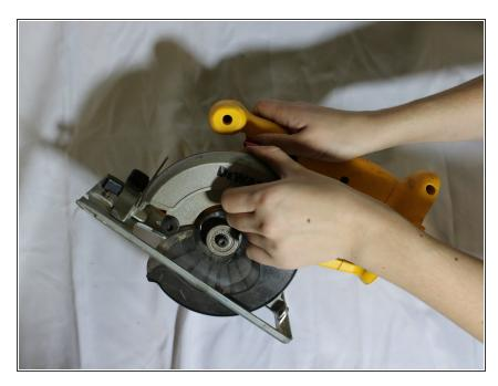
Pull the blade away from the body of the saw causing the blade and boot to detach.
