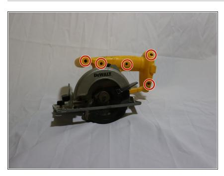
Use a T-15 hexhead screw to unscrew 5 hexagonal screws. These screws are located on the opposite side of the saw from previous step.
