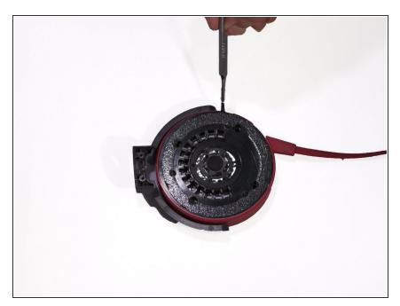
Pry open the front case using the J0 screwdriver.
