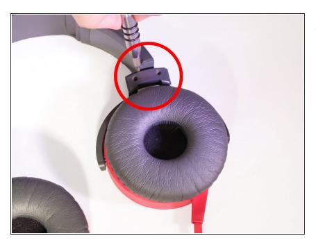
Now that the screws have been removed, pull away the plastic casing that covers the swivel piece (directly above the speaker).
