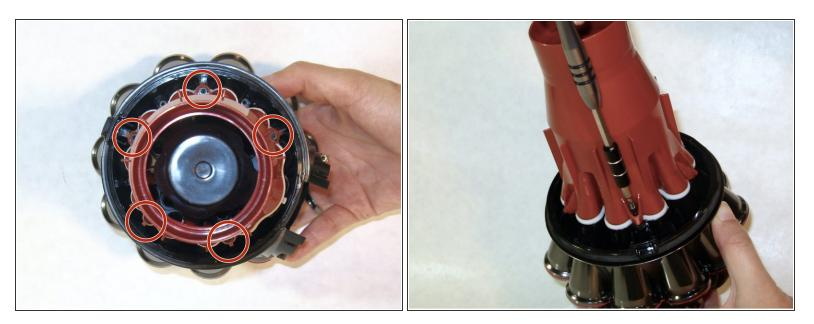
• Use a T9 Torx screwdriver to remove five 14mm screws from the edge of the screen filter body.
