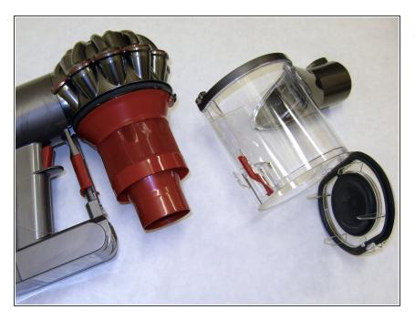
• Separate the bin from the main body of the device.
