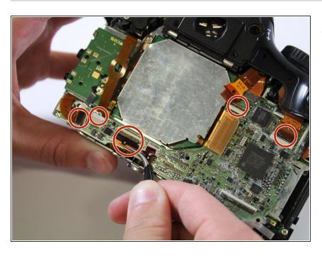
Disconnect the five cables attached to the motherboard by gently pulling with tweezers.
