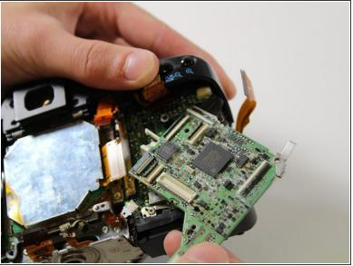
Remove motherboard by gently lifting out with fingers.
