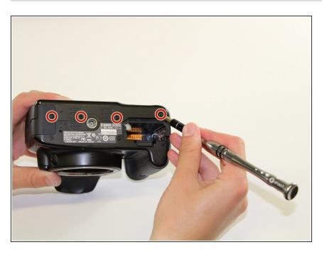
Using the PH000 screwdriver head, remove the four 4 mm screws on the bottom of the camera.
