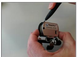
• Gently open the four tabs with a small flathead screwdriver.
