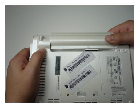
Slide the battery out while holding the left locking tab in the unlocked position.
