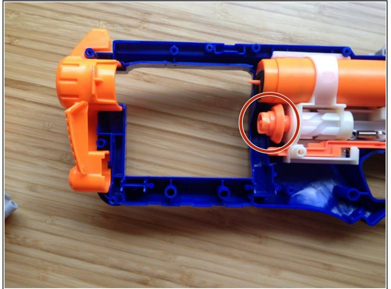
**i** Remove the barrel that holds the Nerf darts.
