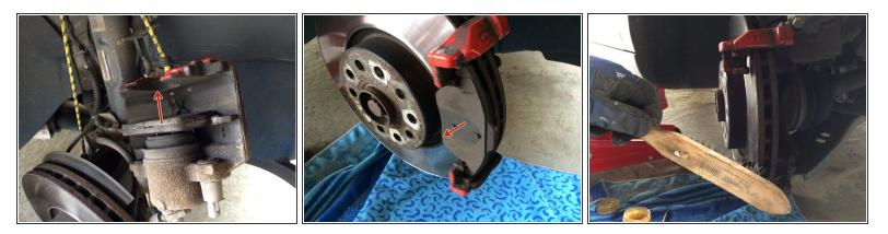
• Hang the removed caliper with a strap, because of the brake hose can be bent. Remove the old brake lining on the piston, this is clipped. Pull off the second brake pad laterally. Then clean the brake with a steel brush.
