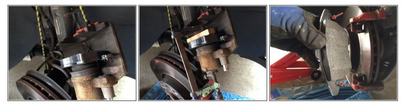
• Click in the new brake pad in the brake piston. With a screw clamp back the whole Bremskoben so that he goes over the pads later. Apply the second brake pad. The running surfaces of the brake pads should be slightly greased.
