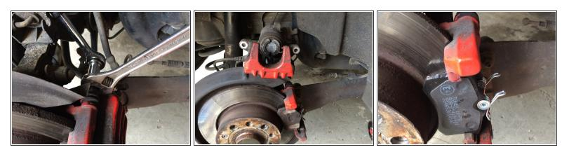
Completely unscrew the brake caliper screws with a 15 mm open-end wrench. Remove brake caliper and remove old brake pads. Then clean the brakes and install new brake pads. Lubricate the treads a little.
