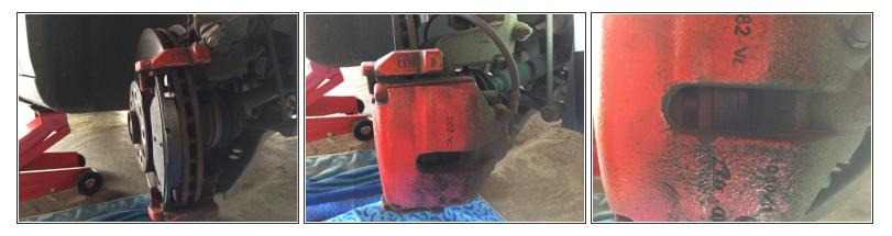
When the pads are in place, replace the brake caliper and tighten. Replace the protective caps.
