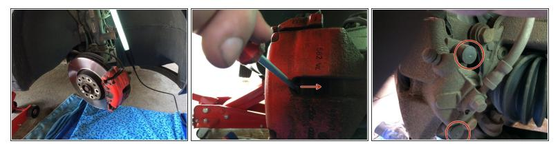
The car must be jacked up with a jack. Then dismantle the wheel in its engaged state. Push back the brake piston with a screwdriver. Remove the two plastic caps on the brake caliper retaining screws
