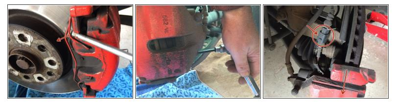
Remove circlip with a screwdriver. Loosen screws with a 7mm Allen key. Then the caliper can be removed by pulling it backwards. If the brake pad has a wear sensor, it must first be removed. Here with a screwdriver behind the lock release.
