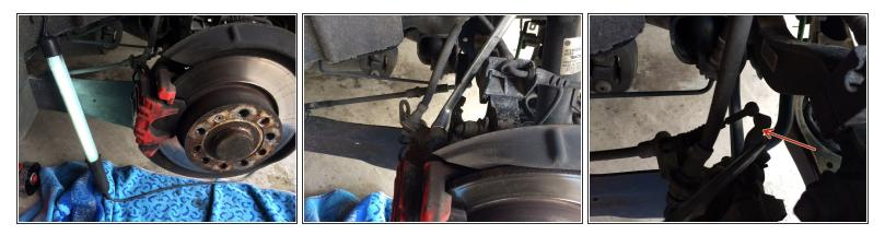
• Jack up the rear of the car and remove the rear wheel. Release brake caliper screws. Unhook the parking brake cable and remove completely to the rear.
